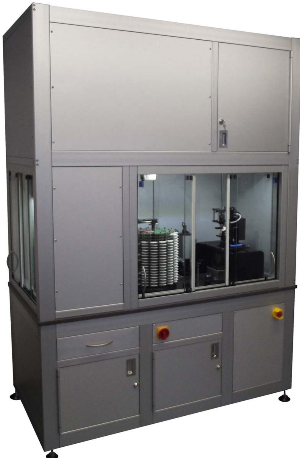
**Automatic weighing system (AWS) used to weigh dust-laden filters with a diameter of 47 mm for registration and documentation of particulate matter (Pat. pend.)**
